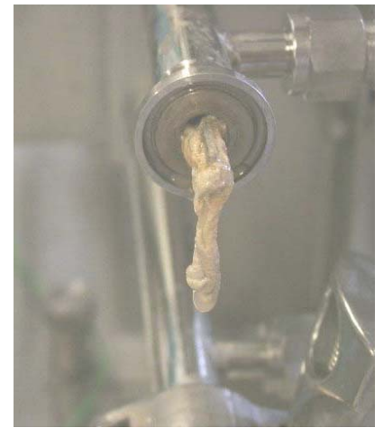
Fig. 3: denaturated protein of control sample without phosphate in UHT facility, pilot plant BK Giulini GmbH, Ladenburg
